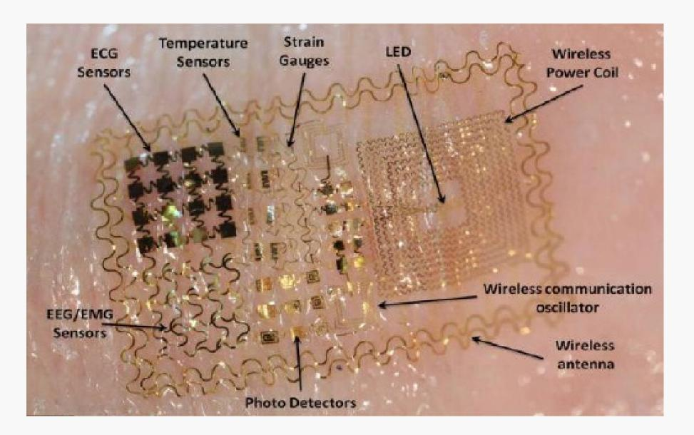
Biostamp use high-performance silicon, can stretch up to 200 per cent and can monitor temperature, hydration and strain, among other medical statistics. Javey's study claims that while building sensors into networks isn't new, interactive displays; being able to recognize touch and pressure and have the flexible circuit respond to it is 'breakthrough'. His team is now working on a sample that could also register and respond to changes in temperature and light to make the skin even more lifelike.
